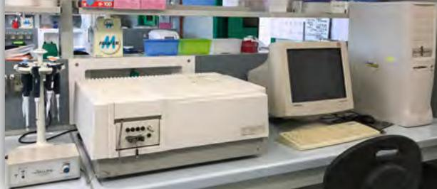
The aim of this training is to monitor, in real-time, the fusion between membranes using a fluorimetric method for assaying membrane fusion exploit processes in a cell-free model system that reflects the final step of exocytosis. Specifically, isolated vesicles are labeled with a lipid-soluble fluorescent probe (octadecylrhodamine R18), at self-quenching concentration and, as a consequence of fusion with unlabelled membrane, lipid probe dilution occurs,
